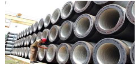
PC Piles Spun & Square (spinning method) and PC Piles Square & Triangle (vibration method).
